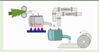
Chemicals / ingredients such as starch and bonding agents are added. The pulp is poured over a fine mesh and the water escapes leaving the cellulose fibres behind. This forms the paper.
