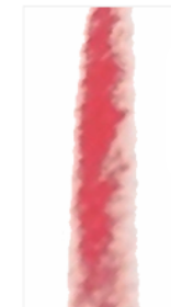
A TYPICAL BLEED LINE ON CARTRIDGE PAPER
